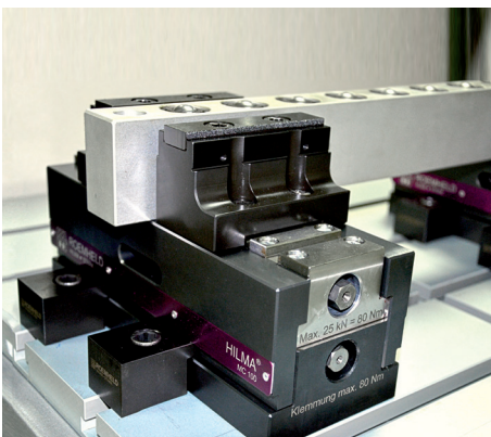
Clamping of aluminium bars with workholding system HILMA.MCP 100 Z Balance.
