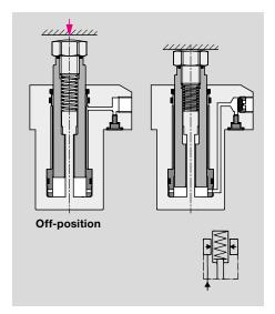
The support plunger is pushed back by the inserted workpiece, the spring force has to be overcome.
