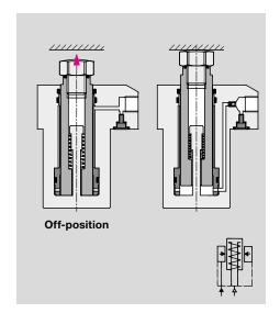
The support plunger contacts the workpiece by air pressure. The contact force is proportional to the air pressure less spring return force. The support plunger will be locked by hydraulic pressure and can compensate forces in axis direction.
