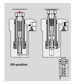
The support plunger is extended by a hydraulically pressurised small piston and contacts the workpiece with spring force.
