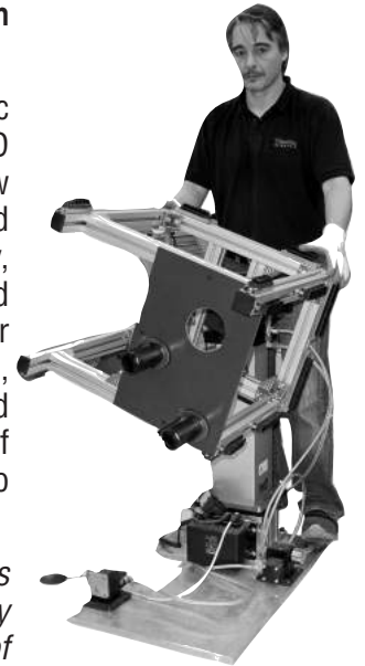
The rotary module has indices which may be released in steps of 45° by two foot switches.
